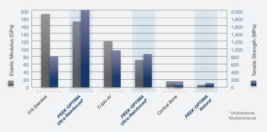
Plates composed of PEEK-OPTIMA Ultra-Reinforced can be designed with a level of stiffness that ranges from lower than titanium to greater than stainless steel.
