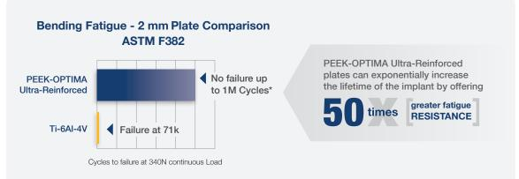
\*While the test was stopped at 1M cycles, the devices didn't fail up to that point.
